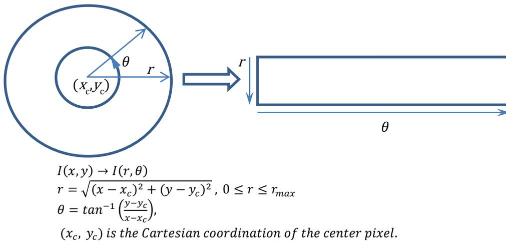
Fig. 7 Daugman Model based normalization process and equations
