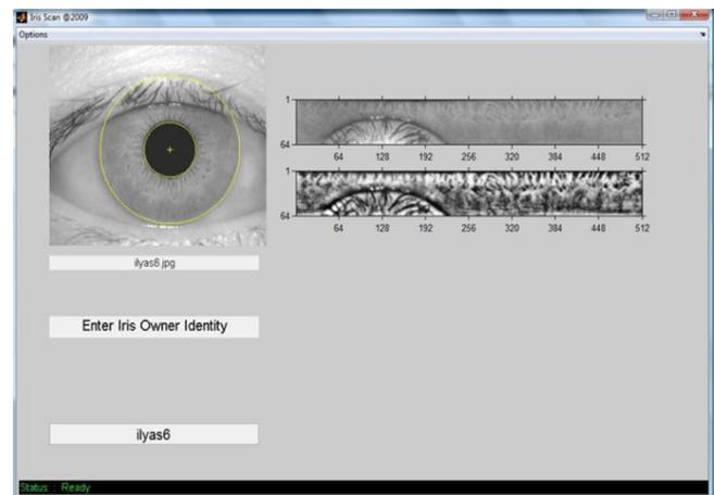
Figure 11 Iris Recognition Implementation in Matlab: IrisScan
