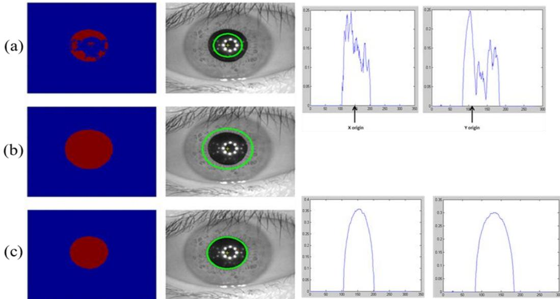
Fig. 5 Iris-Pupil Boundary Localization after MM operations: (a) original, (b) dilation, and (c) erosion
